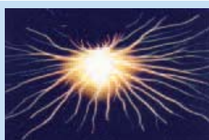
Figure 5: Propagating brush discharge with a relatively high ignition energy (ignition possible when dust is present)
