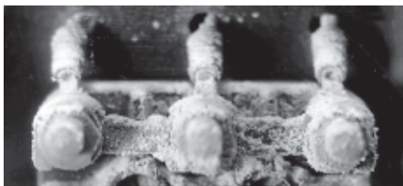
gap 0.05 mm, without gasket, standard talcum powder
