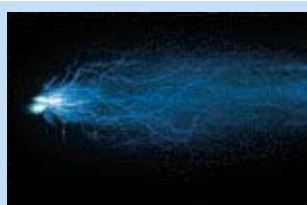
Figure 4: Brush discharge with a relatively low ignition energy (ignition possible when gas is present)
