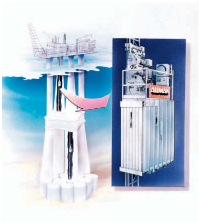
Figure 2: Repair and maintenance elevators inside the supporting steel construction of an offshore platform
