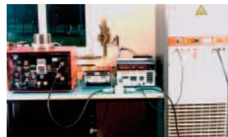
Figure 2: Test set-up for measurement of the ignition limit values for frequencies up to 100 kHz
