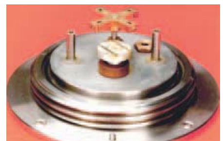
Figure 3: Modified contact arrangement of the spark test apparatus
