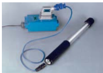
Figure 1: Intrinsically safe lighting device with 8 W fluorescent lamp
