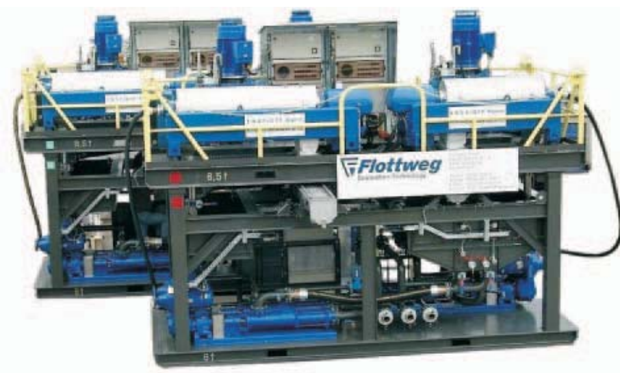
Figure 4: Flottweg barite recovery installation, with sets of two decanters including control systems
