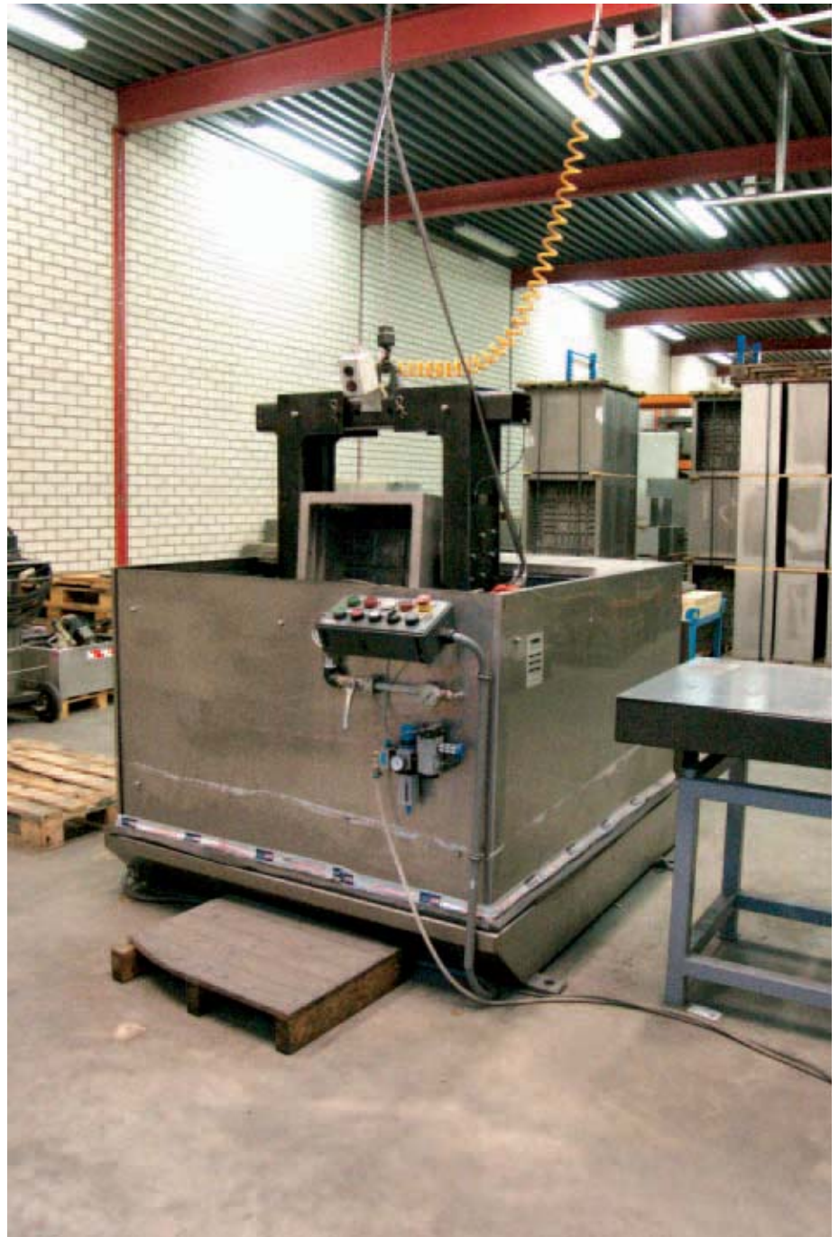
Figure 3: Pressure test device for testing flameproof enclosures (routine test)
