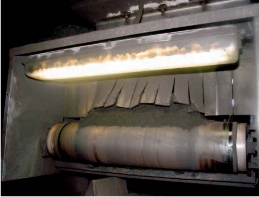
Figure 1: Continuously operating coal sweepers convey 4,000 metric tons of coal every day to the further-processing systems of the HKM coking plant in Duisburg, Germany. Over 400 explosion protected luminaries ensure safe illumination of the uphill and downhill walkways
