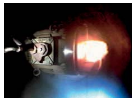
Figure 4: Flame transmission of internal ignition at a shaft gland joint
