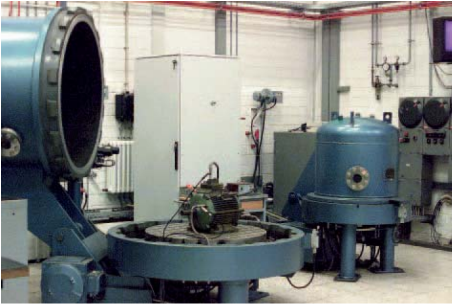
Figure 1: Pressure vessel for testing electrical equipment with type of protection Flameproof enclosure "d"
