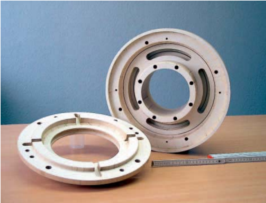
Figure 6: Prototype of a fixture for porous structures for avoidance of flame transmission on rotating electrical machines of large size
