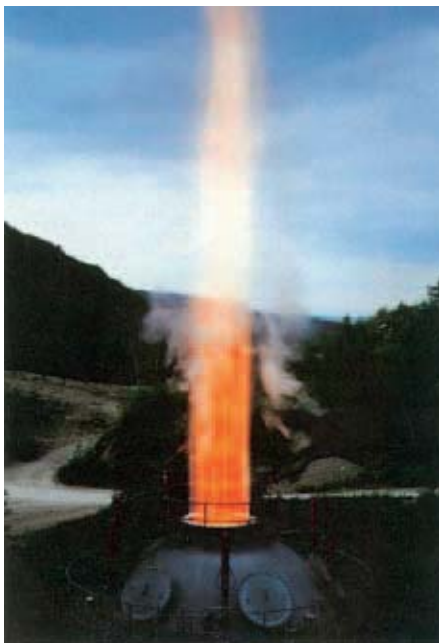
Figure 1: Relief venting rapidly developing dust explosion of a 250 m 3 vessel
