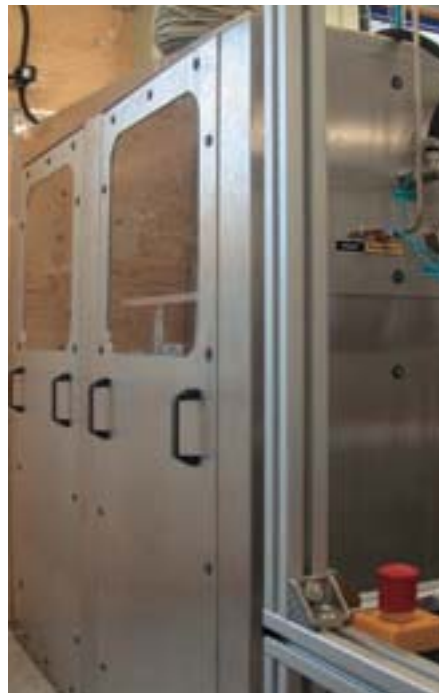
Figure 3: Explosion protection compartment
