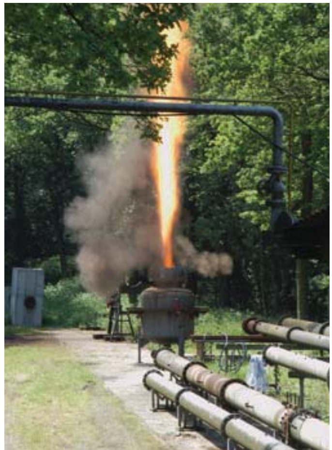
Figure 6: Explosion test on the outdoor test facility in Dortmund-Derne
