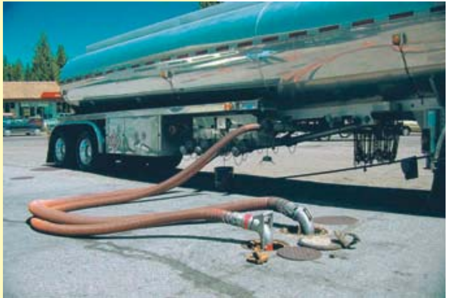
Figure 1: Tank filling operation in a tank farm
