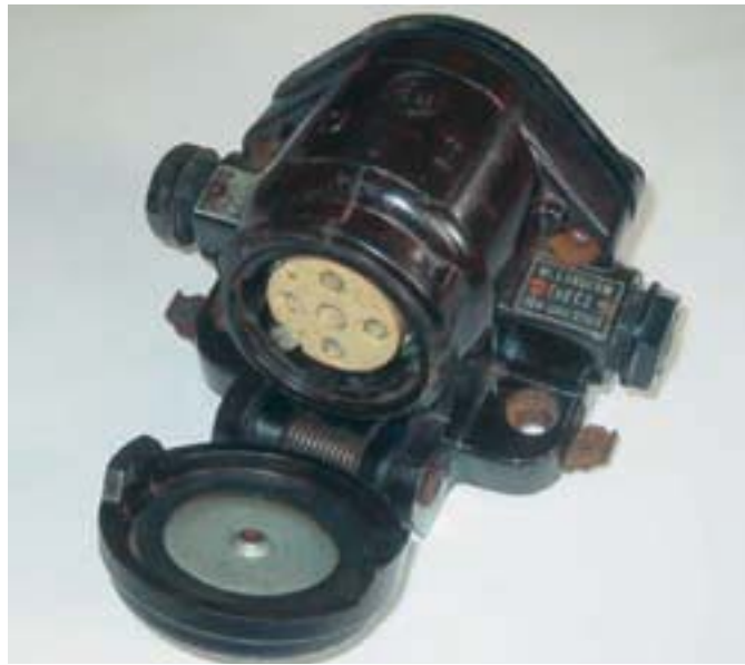
Figure 3: Socket for three phase current type of protection ex d C3 (Marking according to VDE 0171/1.44 V, C = ignition temperature >175 °C, 3 = gap of the joint 0.5 mm; C 2 excluded CS 2 ), enclosure of bakelite, connection chamber ›Ex e‹, flame transmission resistant rotary switch with a ceramic bushing; manufactured by Stotz Kontakt before 1957
