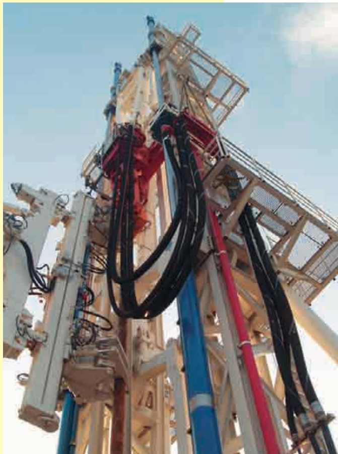
Figure 1: HERRENKNECHT derrick with the pipe handler
