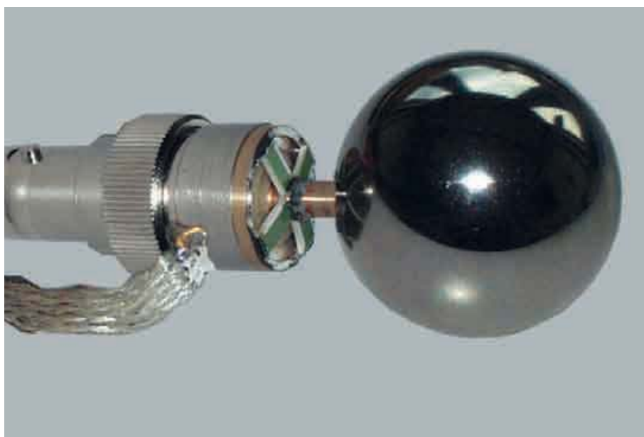
Figure 5: Ball electrode with connected coaxial 0.25 Ohm shunt resistor, attached to the input channel of an oscilloscope
