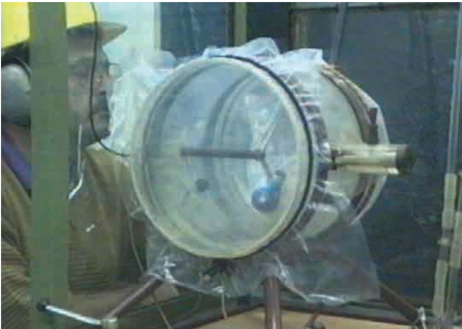
Figure 1: Experimental ignition test to verify the effectiveness of anti-ignition measures
