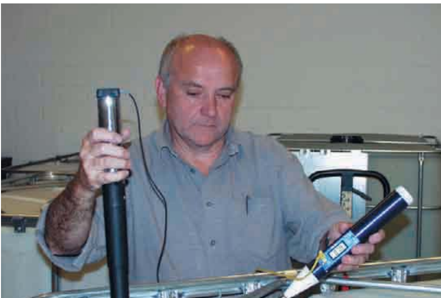
Figure 4: Applying a charge with a needle electrode and then measuring the transferred charge Q with a coulombmeter
