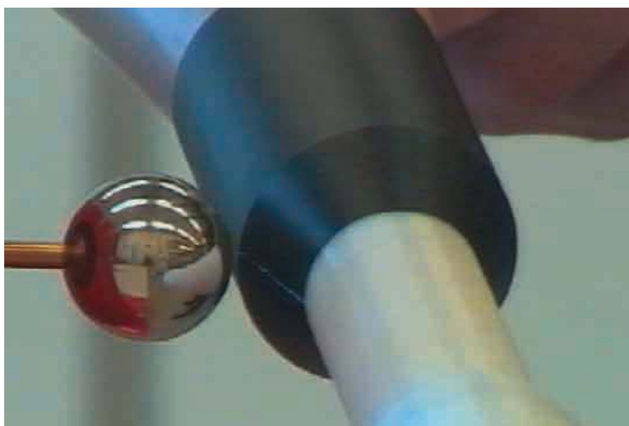
Figure 6: Spark-over from an electrostatic hand-held spray device to the test electrode
