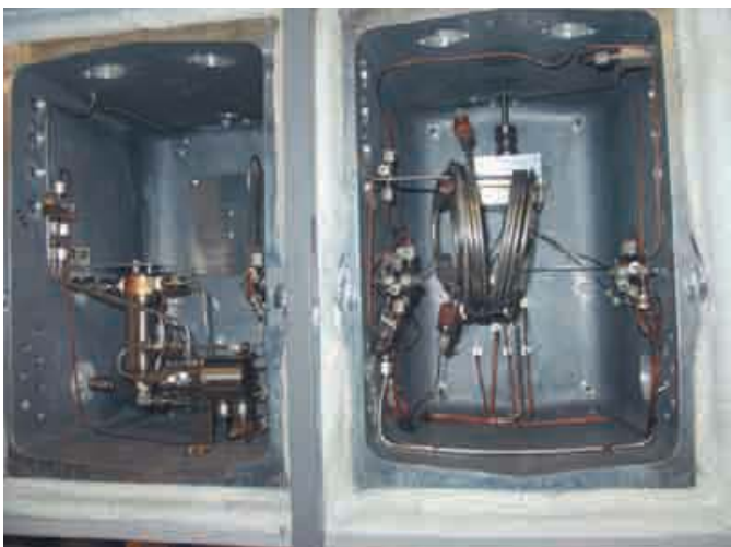
Figure 4: Two oven technology of the process-gas chromatograph Maxum Edition II: detector and sample conditioning are separated into two rooms
