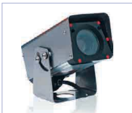
Figure 2: A high-resolution image from hazardous areas is provided by the camera EEx zoom 80 AF, which has an 18/12-times zoom and a night-vision function
