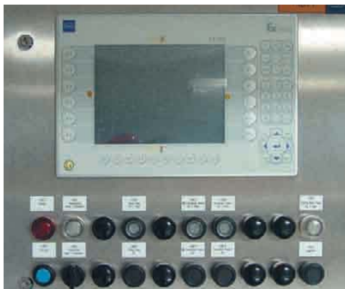
Figure 2: Explosion protected control panel with operator interface ET 306 and discrete controls and indicators
