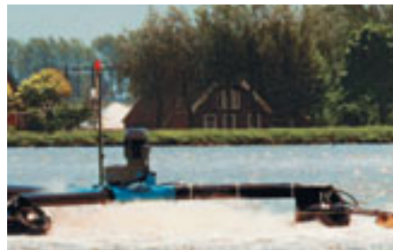
Figure 2: Aerator for increasing the oxygen content of a drinking water tank Continuous operation: 24 h/d (hours per day) 365 d/a (days per year)
