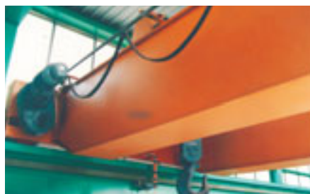
Figure 3: Power station crane for the inspection of turbine and generator Short operation: A few minutes per year
