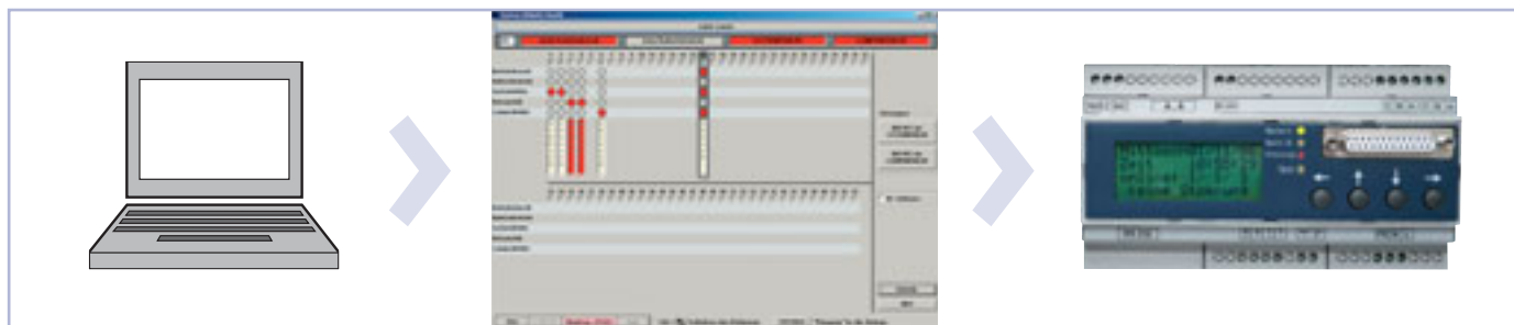
Figure 7: Central unit that enables the central battery system to be individually configured and monitoring tasks to be performed
