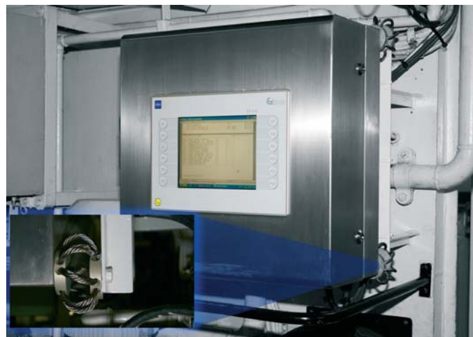
Figure 3: Using buffering mounts at all four corners of the stainless steel housing, typical ship vibration is reduced to protect the electronics of the HMI
