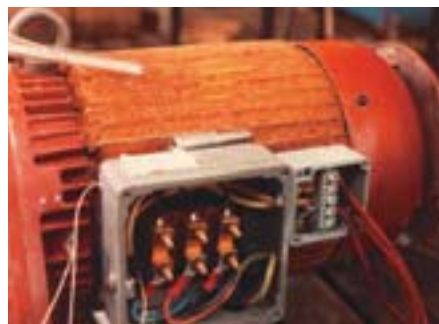
Figure 11: Testing temperature rise with dust covering on the upper side in the case of Practice B (dust blanket test) in accordance with IEC and EN 61241-1 (source: Danfoss Bauer on the occasion of an earlier UL acceptance test)
