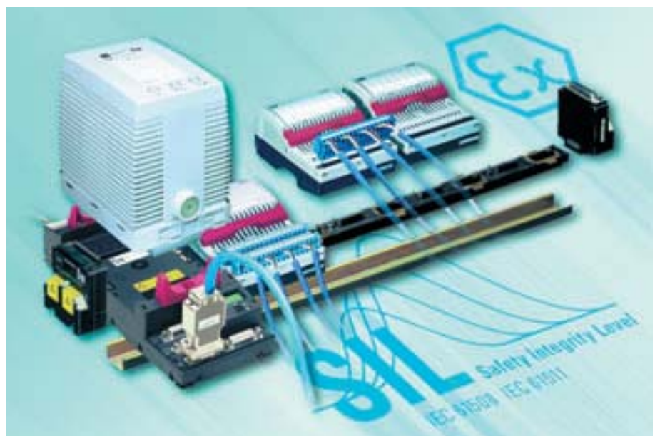
Figure 6: Remote I/O System IS1 for safety requirements up to SIL 1
