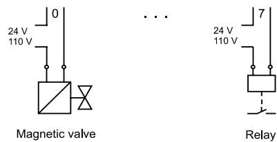
Fig. 7-18 Digital Output Module Relay Type 9477 (connectable field device types)
